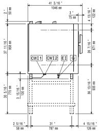
CWI1 = Cold Water inlet 1 (cleaning) CWI2 = Cold Water Inlet 2 (steam
